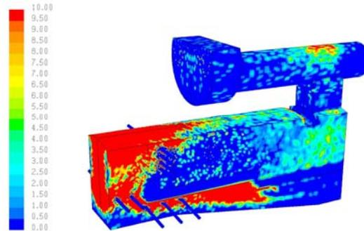
**Figure 5:** Coarse fly ash particle mass flux (deposited particle mass) to furnace and fire tube boiler walls in  $\text{mg}/\text{m}^2\text{s}$ . (Calculation of reference viscosity according to Equation 4)
