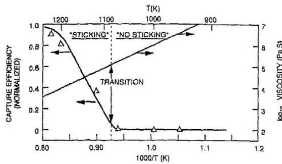
**Figure 1:** Measured capture efficiencies and calculated viscosity as a function of temperature of glass particles ( $53\mu m < d_p < 74\mu m$ ) at a velocity of 4 m/s (source: Srinivasachar et al., 1990)
