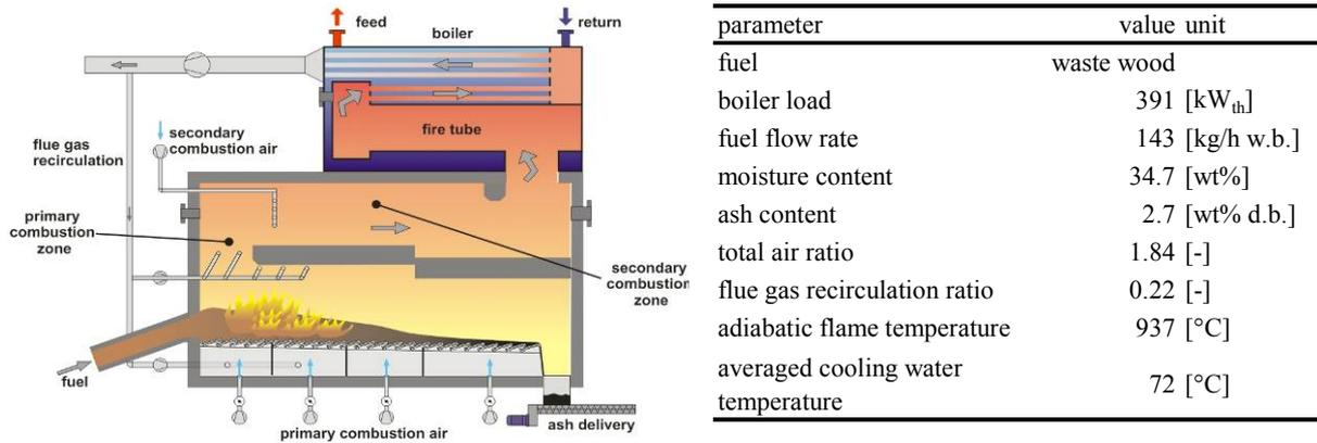
**Figure 3:** Scheme of the biomass combustion plant and operating parameters. The CFD simulation domain of combustion and ash deposition includes the furnace and the radiative section (fire tube) of the boiler. (w.b.: wet base; d.b.: dry base)
