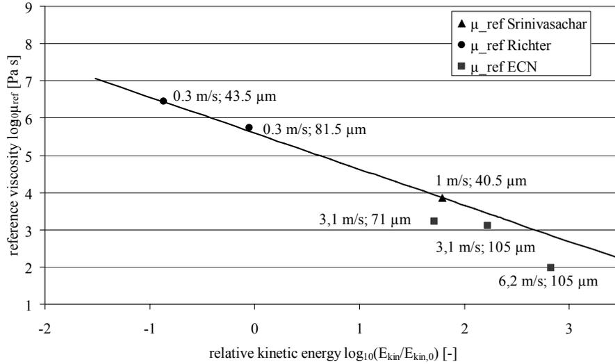
**Figure 11:** Measured reference viscosities  $\mu_{ref}$  as a function of relative kinetic energy
