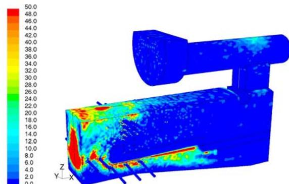
**Figure 9:** Coarse fly ash particle mass flux (deposited particle mass) to furnace and boiler walls in  $\text{mg/m}^2\text{s}$  ( $\mu_{ref} = 10^6$  Pa s)
