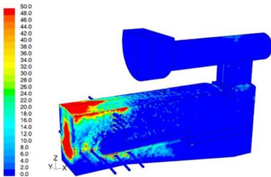
**Figure 8:** Coarse fly ash particle mass flux (deposited particle mass) to furnace and boiler walls in  $\text{mg/m}^2\text{s}$  ( $\mu_{ref} = 10$  Pa s)
