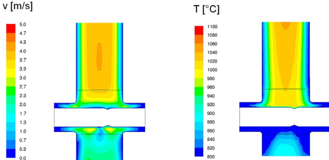
**Figure 14:** Velocity and temperature profiles in the symmetry plane of the reactor tube (case 2,  $T=1015^{\circ}\text{C}$ )
