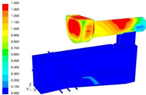
**Figure 4:** Total condensation mass flux of ash forming vapors considered on furnace and fire tube boiler walls in  $\text{mg}/(\text{m}^2\text{s})$
