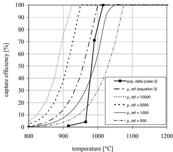
**Figure 18:** Capture efficiency for different reference viscosities in comparison with experimental data (case 2)
