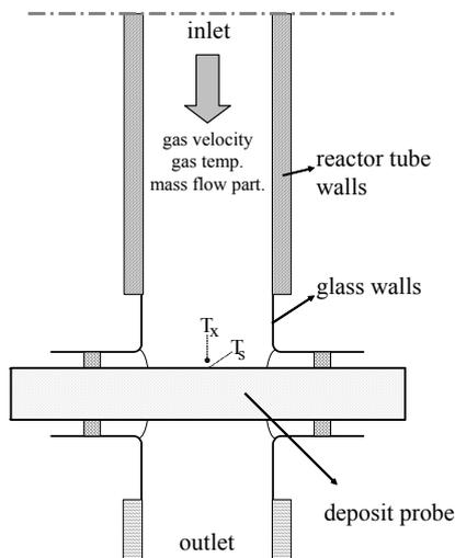
**Figure 10:** Scheme of the lower part of the lab-scale combustion simulator (LCS) of ECN
