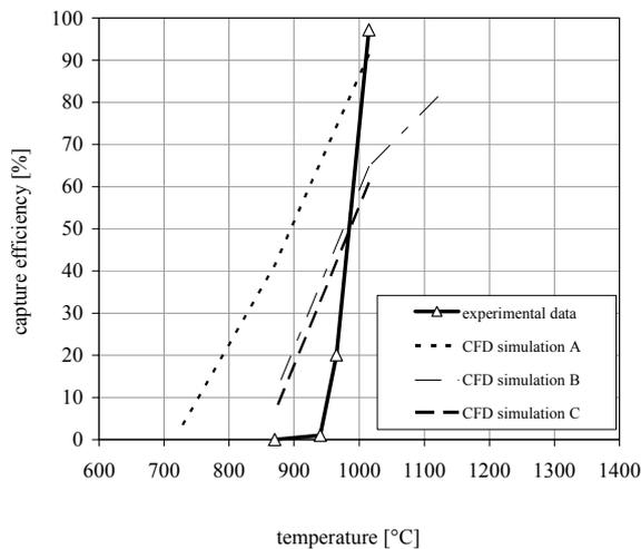
**Figure 17:** Measured capture efficiencies in comparison with CFD-simulated capture efficiencies (simulation A was carried out using a constant temperature field, simulation B taking the normal component for kinetic energy calculation into account and simulation C using the absolute velocity)
