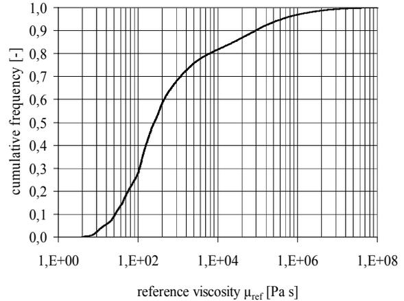
**Figure 7:** Distribution of  $\mu_{ref}$  in the pilot-scale plant for all impacting particles ( $\mu_{ref}$  is a function of kinetic energy, Equation 4). Fraction of deposited mass in the plant is 0.78 (compare Figure 6)
