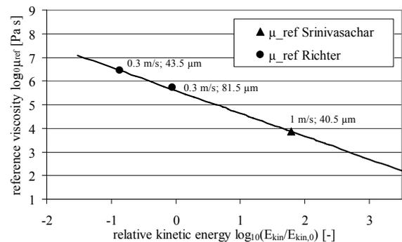
**Figure 2:** Measured reference viscosities  $\mu_{ref}$  as a function of relative kinetic energy of impacting particles ( $E_{kin}$ ...kinetic energy,  $E_{kin,0}$ ...kinetic energy of reference particle source: Srinivasachar et al., 1990; Richter, 2003)
