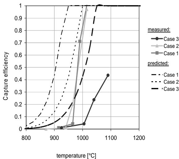
**Figure 12:** Measured and calculated capture efficiencies for 3 different test runs as a function of gas temperatures
