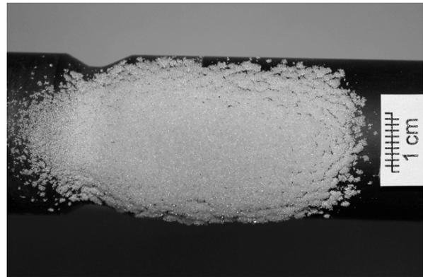
**Figure 13:** Picture of precipitated glass particles on the deposit probe ( $d_p = 71 \mu\text{m}$ ,  $v_p = 3.1 \text{ m/s}$ ,  $T = 10^\circ\text{C}$ )
