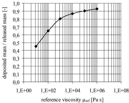
**Figure 6:** Fraction of deposited mass by coarse fly ash particles in the furnace and fire tube as a function of reference viscosities  $\mu_{ref}$  (constant values)
