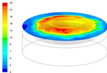
**Figure 10:** Contours of CO concentrations approximately at the surface of the fuel bed [vol%-dry]
