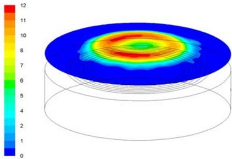
**Figure 9:** Contours of CH<sub>4</sub> concentrations approximately at the surface of the fuel bed [vol%-dry]
