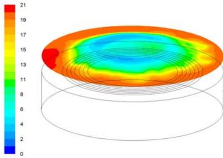
**Figure 7:** Contours of O<sub>2</sub> concentrations approximately at the surface of the fuel bed [vol%-dry]
