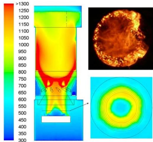
**Figure 6:** Contours of flue gas temperatures (K); left: along the vertical cross section of the combustion chamber; right top: visual observation from a window at the top of the furnace; right bottom: along a horizontal cross section close to the surface of the fuel bed (4cm above the grate, shown in the vertical cross section)
