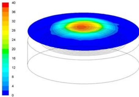
**Figure 8:** Contours of H<sub>2</sub>O concentrations approximately at the surface of the fuel bed [vol%]
