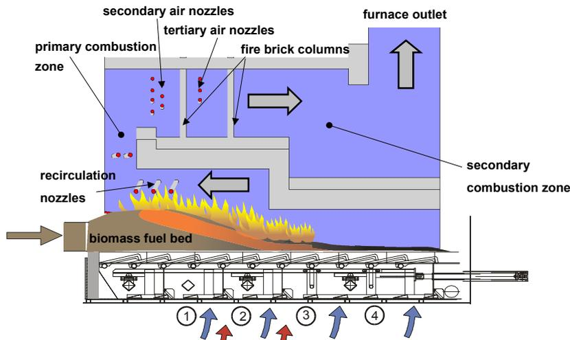
**Figure 9:** Concept of an optimised Multifuel-Low-NO<sub>x</sub> biomass grate furnace
