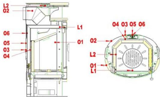
**Figure 8:** Measurement points of surface temperature (O) and air temperature (L) of the basic geometry
