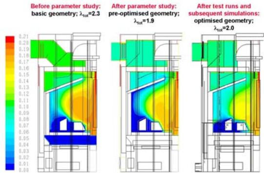
**Figure 12:** Selected results: iso-surface of O<sub>2</sub> concentrations [m<sup>3</sup> O<sub>2</sub>/ m<sup>3</sup> flue gas w.b.] in the flue gas in the vertical symmetry plane of the stove
