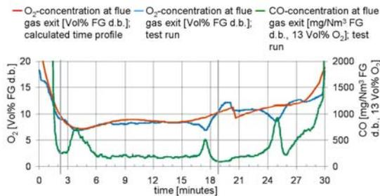
**Figure 5:**  $O_2$  concentrations as a function of time measured in the chimney during test runs (blue curve) in comparison with the calculated  $O_2$  concentrations (red curve), as well as measured CO emissions (green curve); (FG = flue gas)
