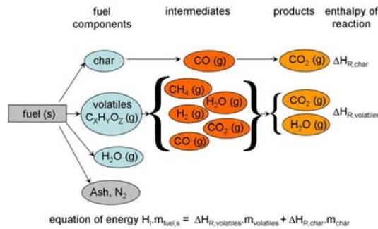
**Figure 4:** Scheme of reactions considered and model for the release of volatiles during wood log combustion; solid fuel components considered: volatiles ( $C_xH_yO_z$ ), vapour from drying ( $H_2O$ ) and char; N-species were released as  $N_2$ ; release rates are source terms in the CFD simulations
