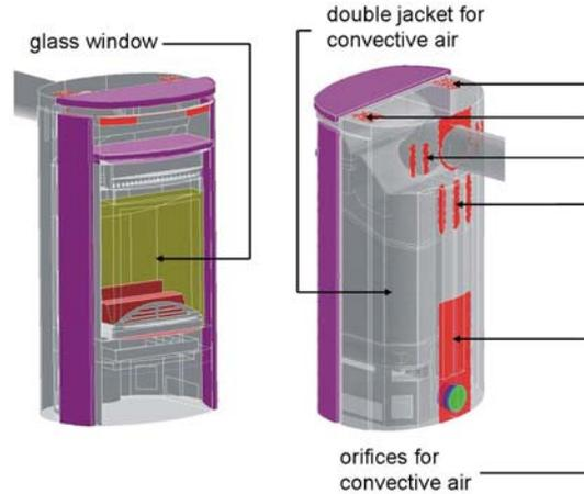
**Figure 2:** Geometry of the wood log fired stove
