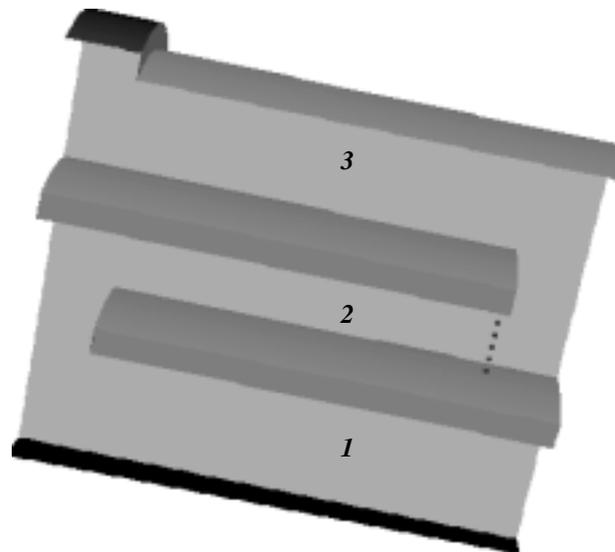
**Figure 4:** Modelled part of the combustion chamber No. 1 (Low-NO<sub>x</sub> furnace, nominal boiler capacity 440 kW<sub>th</sub>)
