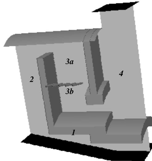
**Figure 5:** Modelled part of the combustion chamber No. 2 (Low-NO<sub>x</sub> furnace, nominal boiler capacity 550 kW<sub>th</sub>)
