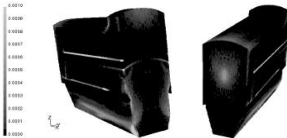
**Figure 7:** Calculated erosion rates [kg/m<sup>2</sup>s] for the combustion chamber walls
