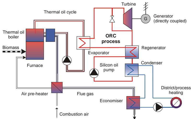
Figure 4. Schematic illustration of a biomass CHP plant based on ORC technology
