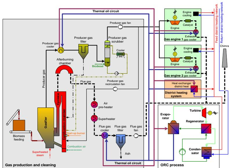
Figure 18. Simplified process scheme of the biomass CFB steam gasification process with integrated gas engines and an ORC unit
