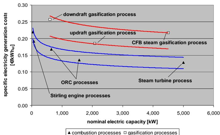
Figure 20. Electricity generation costs for different CHP technologies versus electric power output
