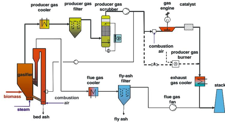
Figure 17. Simplified process scheme of the CFB steam gasification process in Güssing (A)
