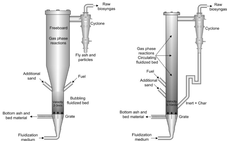
Figure 10. Schematic illustration and operating principle of fluidised bed gasifiers
