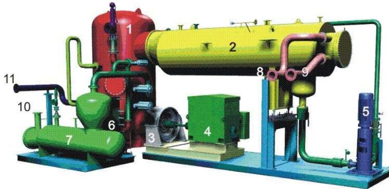
Figure 3. Schematic illustration of a 1,000 kW<sub>el</sub> ORC module
