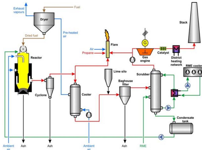
Figure 12. Process scheme and operating principle of the Pyroforce technology
