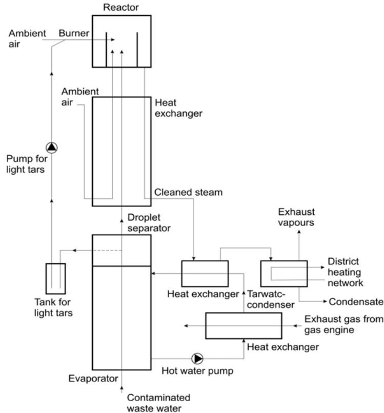
Figure 13. Simplified flow sheet of the TARWATC-process
