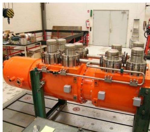
**Figure 1:** Picture of the 75 kW<sub>el</sub> Stirling engine (Stirling engine heater not mounted)
