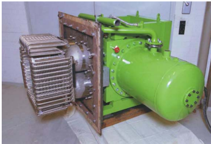
Figure 2: 35 kW Stirling engine before installation in the furnace
