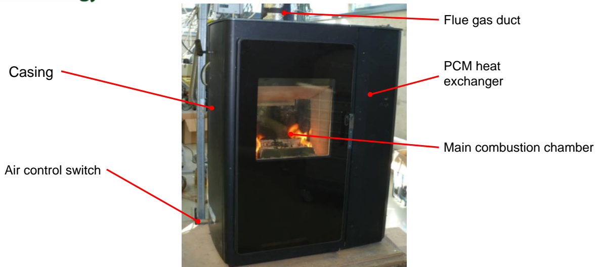
Figure 8: Picture of the new stove technology with integrated heat storage unit based on PCM (the new stove concept is protected by a patent) (source: RIKA)
