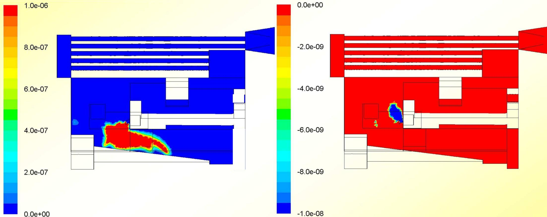
Iso-surfaces of the reaction rates [ $\text{kmol}/(\text{m}^3 \cdot \text{s})$ ] of the reaction  $N + NO \rightarrow N_2 + O$  for the reduction to  $N_2$  (left) and of the reaction  $N + NO \leftarrow N_2 + O$  for the formation of NO from  $N_2$  (right) in the symmetry plane of the combustion chamber and the boiler
