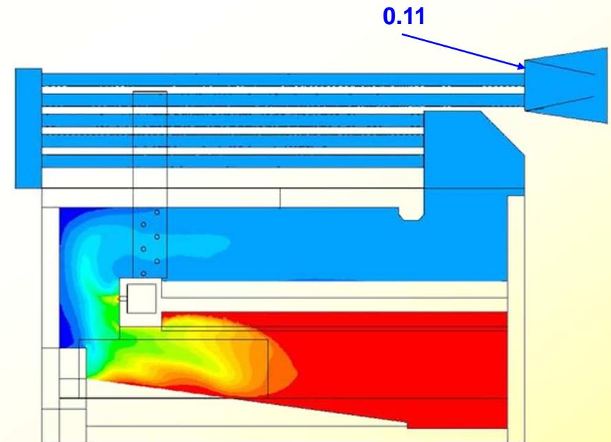
**Iso-surfaces of local TFN/TFN<sub>in</sub> ratios in the symmetry plane of the combustion chamber and the boiler**
