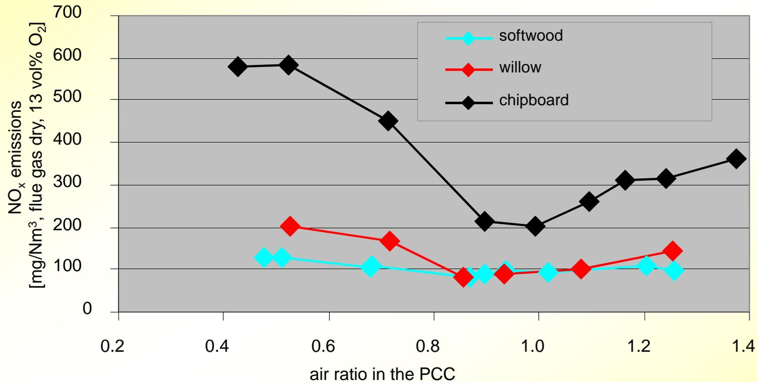
$\text{NO}_x$  as  $\text{NO}_2$  related to dry flue gas and 13vol%  $\text{O}_2$ ; all measurements at full load;
