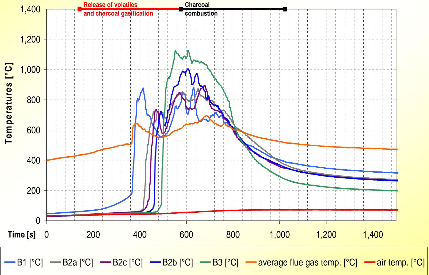
Average flue gas temperature: measured above the fuel bed before reactor outlet
