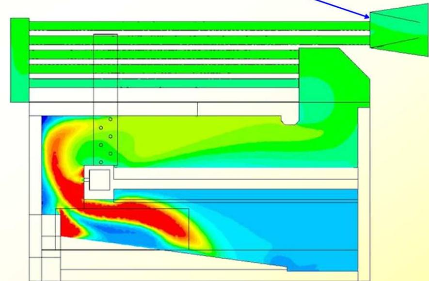
Iso-surfaces of NO<sub>x</sub> concentrations [ppmv w. b.] in the symmetry plane of the combustion chamber and the boiler
