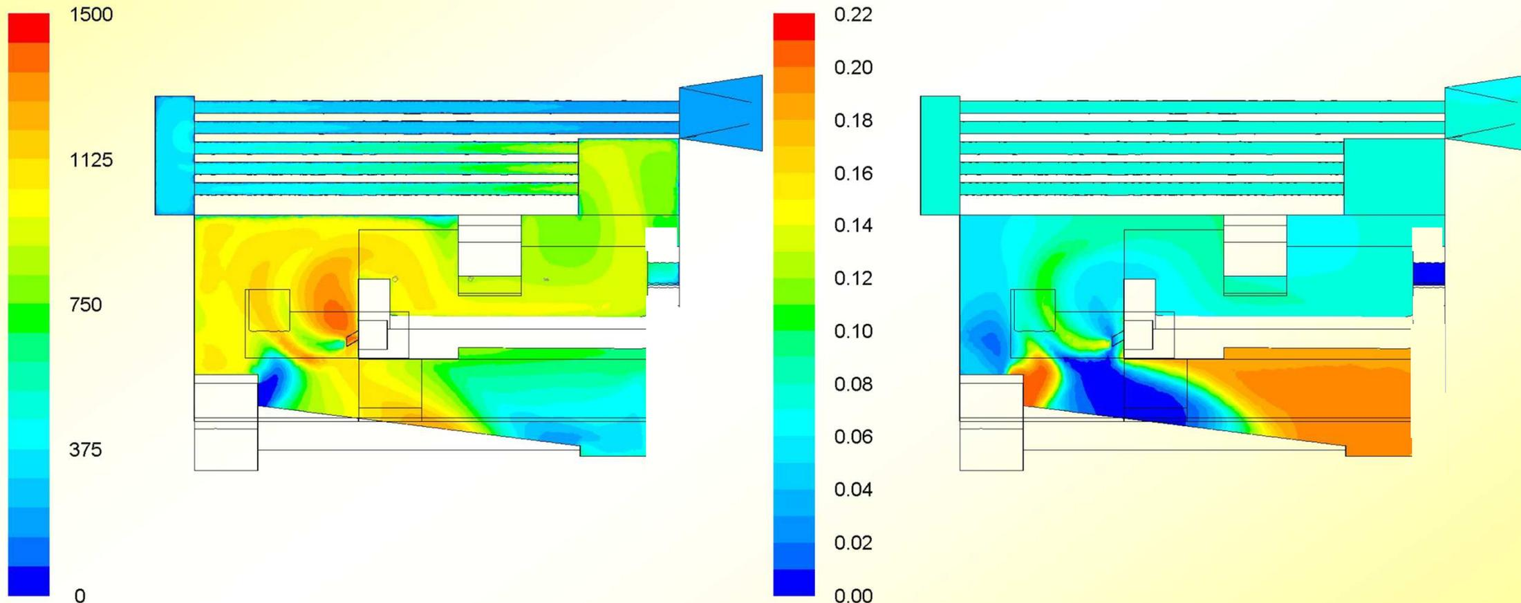
Iso-surfaces of temperatures [°C] (left) and O<sub>2</sub> concentrations [m<sup>3</sup> O<sub>2</sub>/ m<sup>3</sup> wet flue gas] (right) in the symmetry plane of the combustion chamber and the boiler
