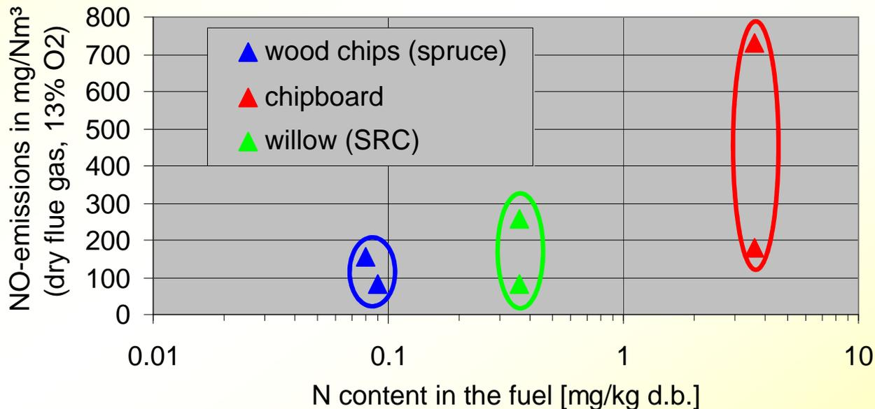
Range of NO<sub>x</sub> emissions at different operation conditions
