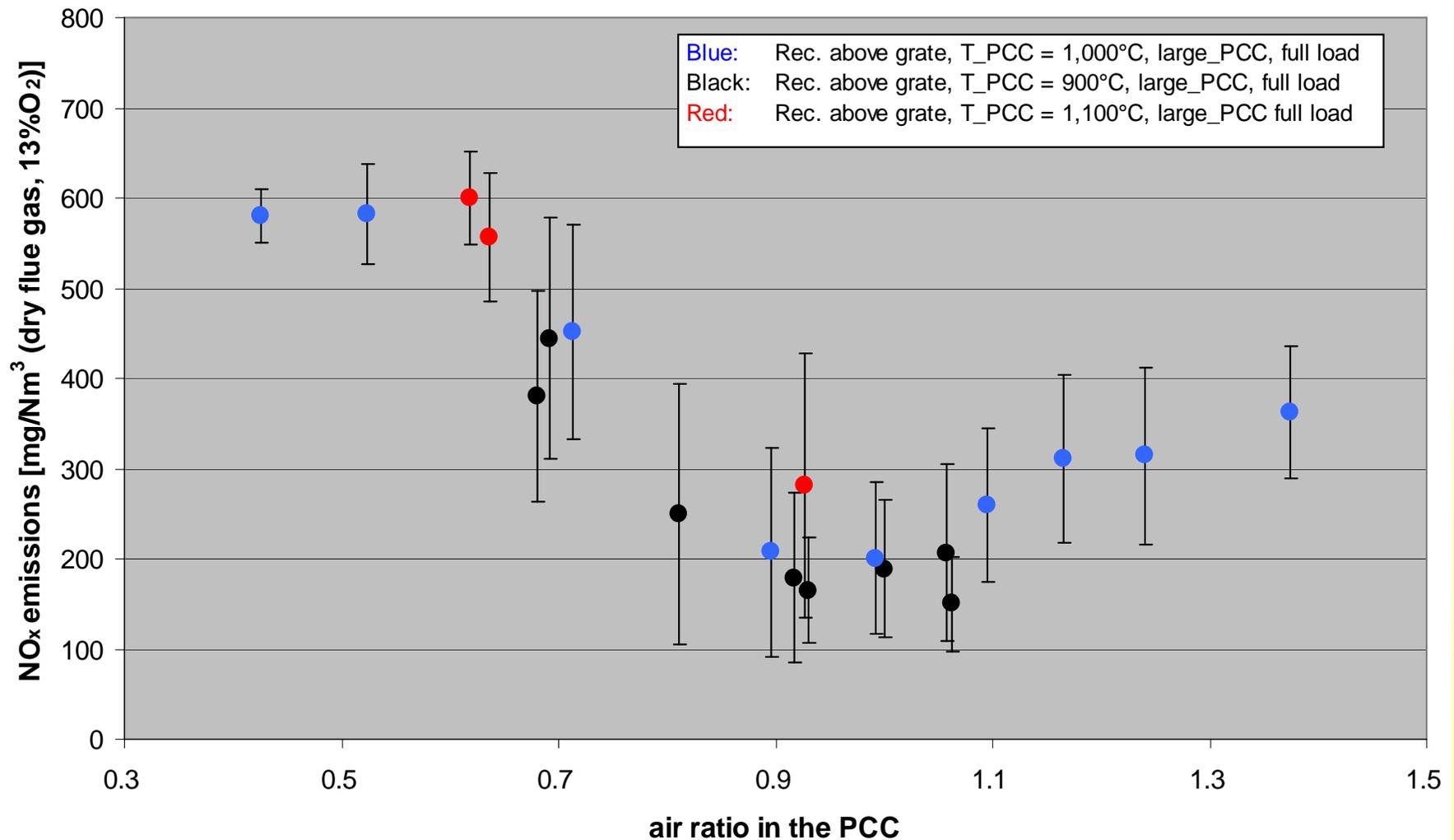
Explanations: Rec ... flue gas recirculation; PCC ... primary combustion chamber;
