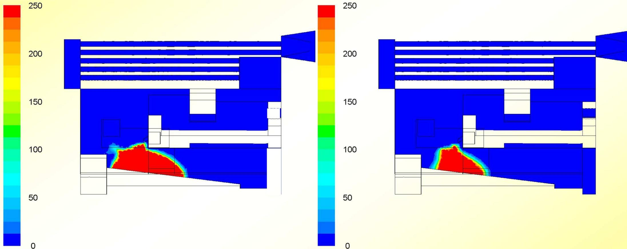
Iso-surfaces of  $\text{NH}_3$  concentrations [ppmv w.b.] (left) and HCN concentrations [ppmv w.b.] (right) in the symmetry plane of the combustion chamber and the boiler
