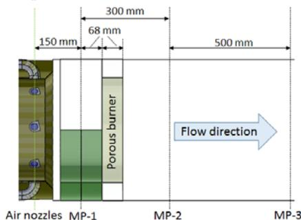
**Figure 4:** Description of the measuring planes upstream and downstream of the porous burner
