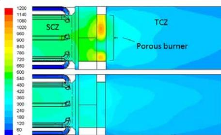
**Figure 9:** Incident radiation [ $W/m^2$ ] in a centre cut through the burner with activated (top) and de-activated (bottom) porous burner model
