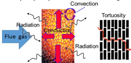
**Figure 1:** Heat transfer mechanisms inside porous burners (left); schematic explanation of a tortuous path through a porous medium.
