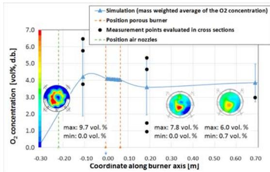
**Figure 11:** Measured  $O_2$  concentrations compared to simulated average  $O_2$  concentrations in the measurement planes
