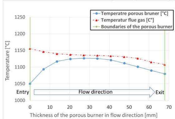
**Figure 8:** Average simulated PIM and flue gas temperatures inside the porous burner evaluated on eleven section planes in flow direction through the porous zone
