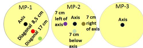
**Figure 5:** Description of the positions of the particular measuring points MP-1 to MP-3
