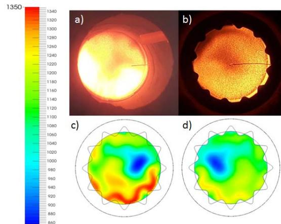
**Figure 6:** a): porous burner seen from the SCZ; b): porous burner seen from the TCZ; surface temperatures of the porous burner according to CFD: c): burner inlet; d): burner outlet.
