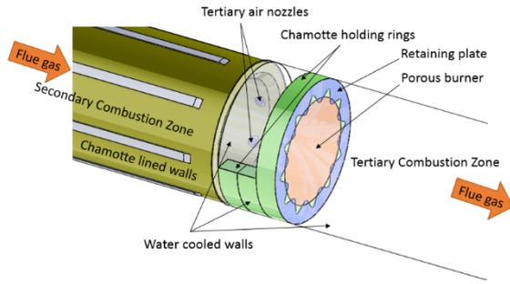
**Figure 3:** 3D geometry of the section where the porous burner is implemented in the burnout zone
