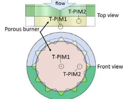
**Figure 7:** Temperature measurement positions in the porous burner: T-PIM1: centre of the outlet surface of the PIM; T-PIM2: in the core of the burner about 5 cm from the edge.
