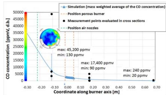
**Figure 12:** CO measurements compared to simulated average CO concentrations including the standard deviations in the measurement planes evaluated
