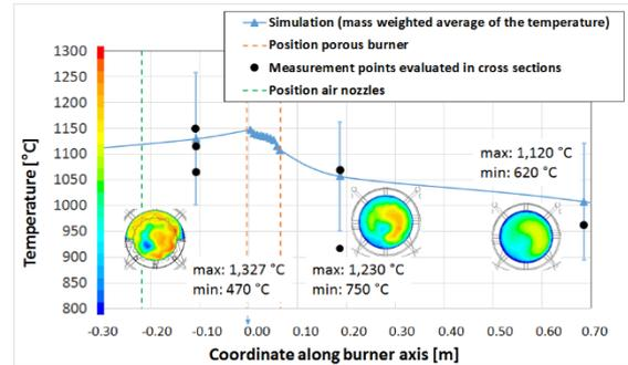
**Figure 10:** Temperature measurements compared to simulated average temperature values in the measurement planes.
