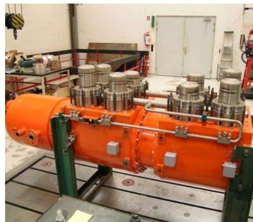
Figure 1: Picture of the 75 kW el Stirling engine (Stirling engine heater not mounted)
