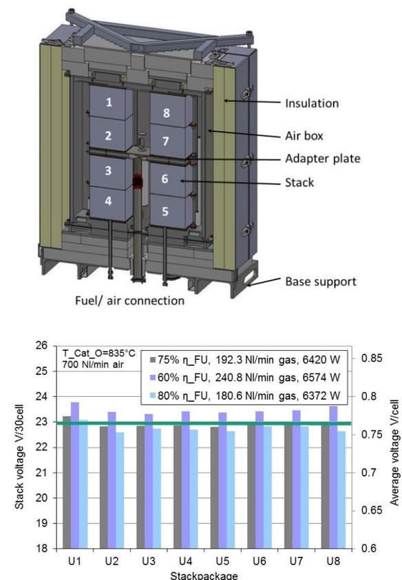
**Figure 3:** Results from performance tests with the stack module with simulated product gas at 35 A
