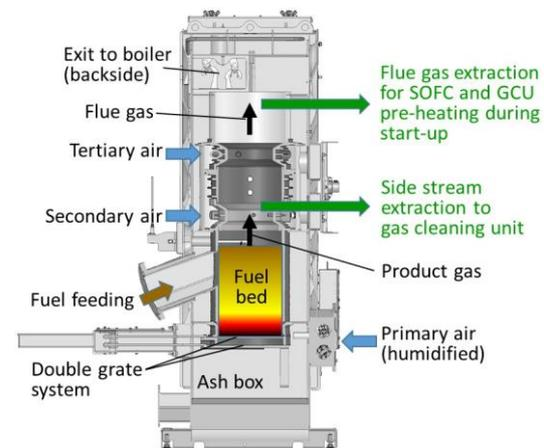
**Figure 2:** Scheme of the fuel-flexible gasifier developed and interfaces to GCU and SOFC units
