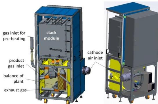
**Figure 4:** Sketch of the SOFC system
