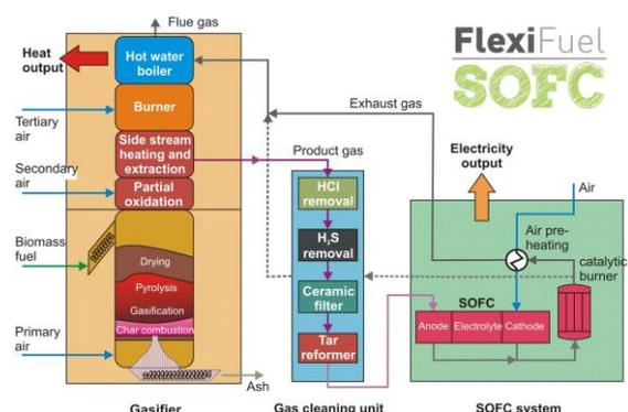
**Figure 1:** Basic scheme of the novel micro-scale air biomass CHP technology
