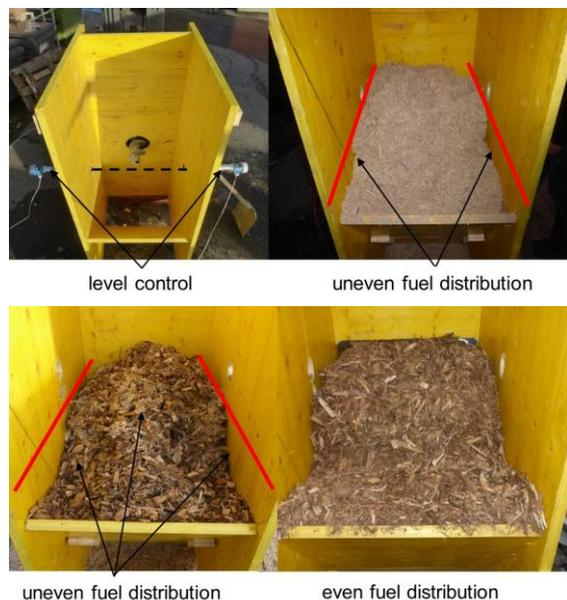
**Figure 3:** Test run set-up for fuel feeding tests with a cold model of the stoker screw and the gasifier fuel bed region
