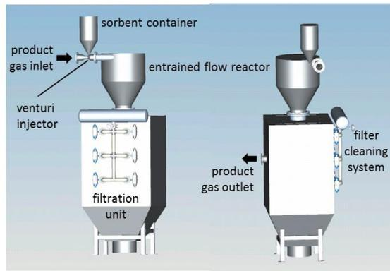
**Figure 6:** Scheme of the gas cleaning unit
