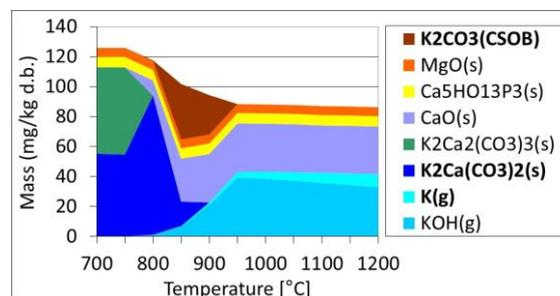
**Figure 4:** Results of thermodynamic high-temperature equilibrium calculations regarding ash formation in the updraft gasifier when utilising wood chips
