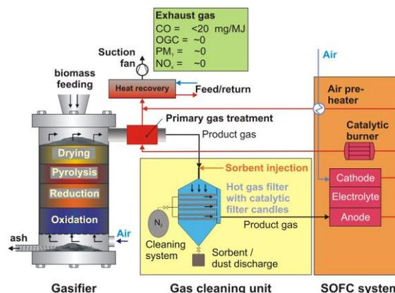
**Figure 1:** Scheme of the HiEff-BioPower technology
