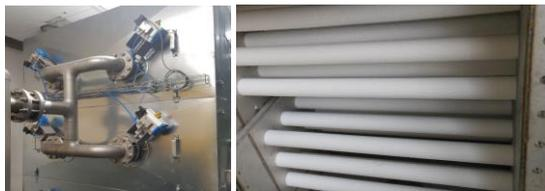
**Figure 7:** Filter cleaning system (left) and view on the ceramic filter candles (right)
