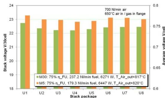
**Figure 10:** Stack module performance
