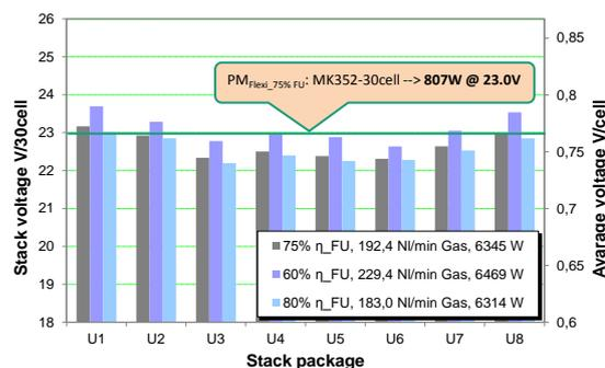
**Figure 7:** 8x30-cell MK352 stack module performance at 845 °C, 35 A at different fuel utilization rates compared to the performance of the single MK352 30-cell stacks
