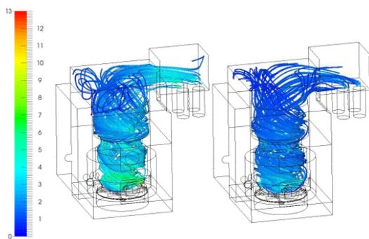
**Figure 5:** Pathlines of the secondary air, coloured by the absolute velocity [m/s] – 3D-view
