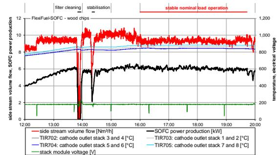
**Figure 15:** Trends of an exemplary operation of the SOFC at nominal load
