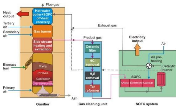
**Figure 1:** Basic scheme of the FlexiFuel-SOFC micro-scale biomass CHP technology
