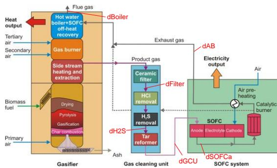
**Figure 2:** Measurement positions for gas sampling
