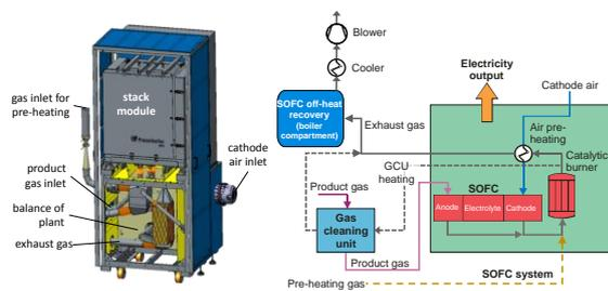
**Figure 8:** 3D model and scheme of the SOFC system (AVL) with integrated stack module (IKTS)
