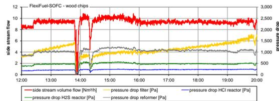
**Figure 10:** Trends of the side stream volume flow and pressure drops of the single units of the GCU
