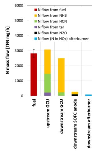
Figure 20: Calculated mass flows of N compounds from the fuel over GCU and SOFC
