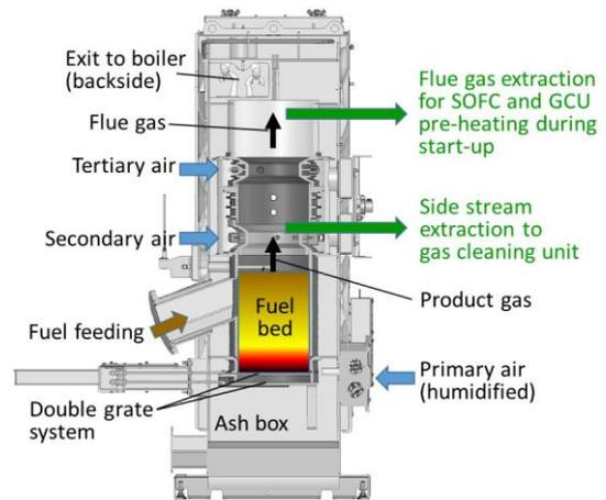
**Figure 3:** Scheme of the gasifier (WHtech) with interfaces to the CHP system
