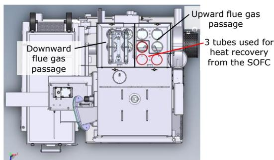
**Figure 6:** Heat recovery from the SOFC off-gas in the boiler
