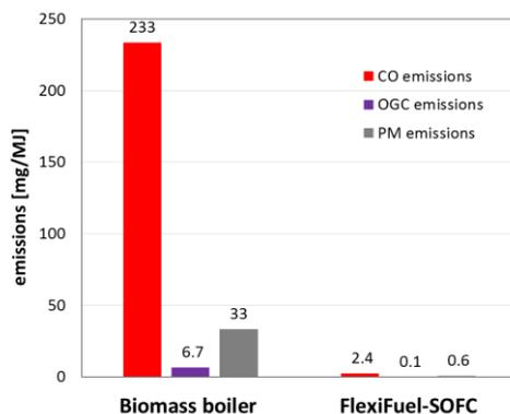
Figure 19: CO, OGC and PM emissions in comparison to conventional biomass boiler systems
