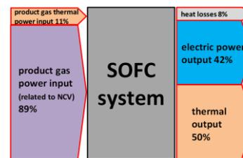
**Figure 16:** Energy balance of the SOFC system at nominal load operation
