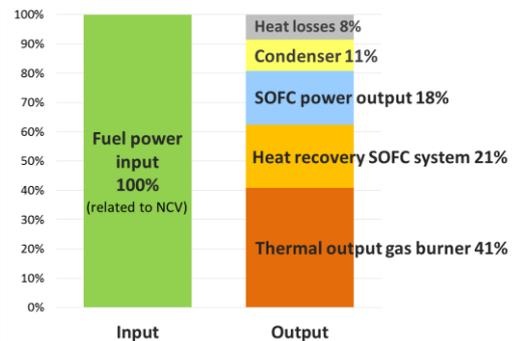
**Figure 17:** Energy balance for CHP operation at nominal load
