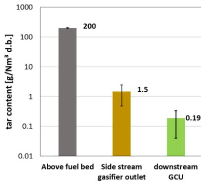
**Figure 14:** Measured gravimetric tar contents of the product gas above fuel bed and of the side stream at gasifier outlet and downstream GCU
