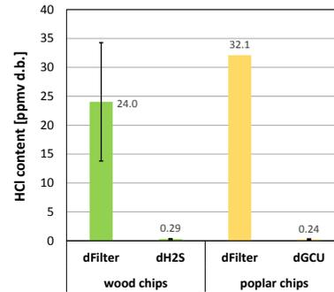
**Figure 12:** Results of wet chemical HCl measurements
