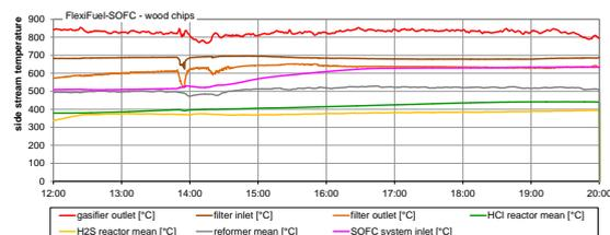
**Figure 11:** Side stream - temperature trends over the GCU
