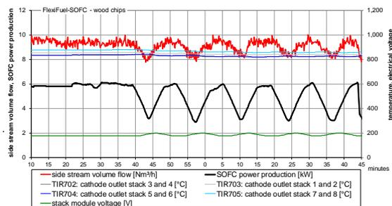
Figure 18: Exemplary trends of load changing tests
