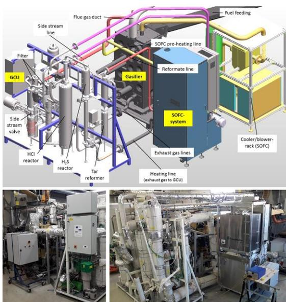
**Figure 9:** 3D model and photos of the testing plant at BIOS in Graz
