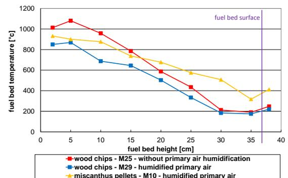
**Figure 4:** Fuel bed temperatures with and without primary air humidification for different fuel moisture contents
