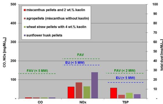
**Figure 15:** Emission of the testing plant in comparison to relevant emission limits
