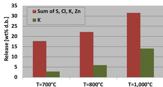
**Figure 5:** Release of K from the fuel bed as a function of the fuel bed temperatures
