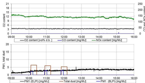
**Figure 11:** Trend of the  $\text{O}_2$ , CO and  $\text{NO}_x$  contents in the flue gas as well as of particulate emissions during a test run with wheat straw pellets with kaolin
