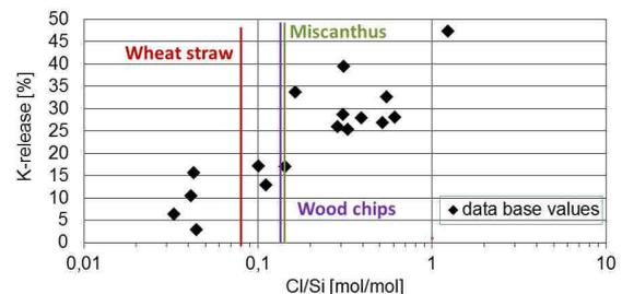
**Figure 2:** K-release rates of herbaceous fuels and chemically untreated wood fuels in dependence of the molar Cl/Si ratio in state-of-the-art grate-fired boilers
