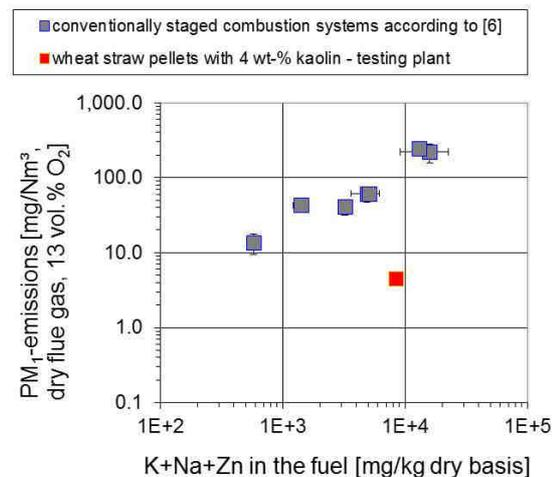
**Figure 13:** Correlation between the concentrations of aerosol forming elements in the fuel (K, Na, and Zn) and aerosol emissions downstream the testing plant
