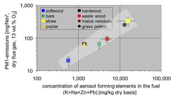
**Figure 4:** PM<sub>1</sub> emissions versus the concentration of aerosol-forming species (K + Na + Zn + Pb) in the fuel
