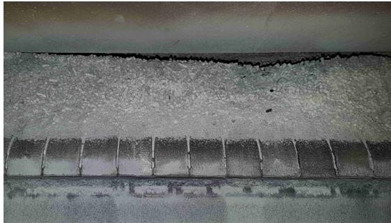
**Figure 14:** Pictures of the grate and ashes from the test run with wheat straw and kaolin
