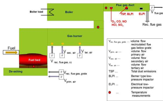
**Figure 10:** Scheme of the testing plant and the measurement set-up for test runs
