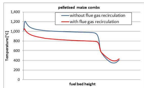
**Figure 7:** Axial profiles of fuel bed temperatures – bed cooling by addition of recirculated flue gas to primary air
