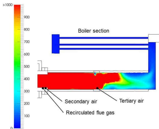
**Figure 8:** Design of the gas burner – optimisation of flue gas burnout
