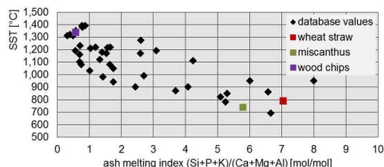
**Figure 1:** Qualitative evaluation of miscanthus, wheat straw and wood chips based on the ash melting index
