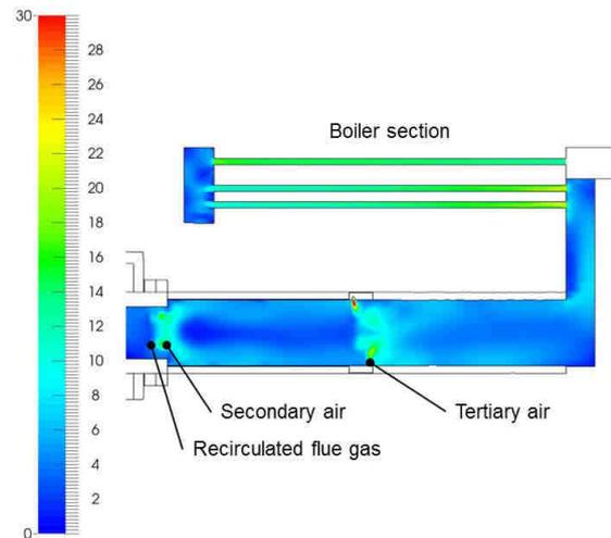
**Figure 9:** Design of the two-stage gas burner – mixture of combustion air with flue gas
