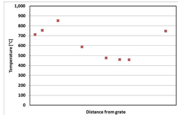
**Figure 12:** Temperature profile of the fuel bed during a test run with wheat straw pellets and kaolin
