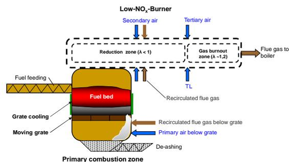
**Figure 6:** Basic concept of the new fuel flexible and low emission combustion technology
