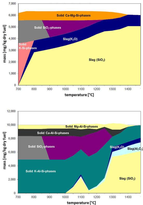
**Figure 3:** The effects of kaolin addition to wheat straw on ash and slag formation – results from TEC
