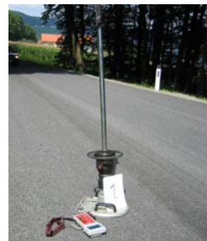
Figure 3: Light falling deflectometer
