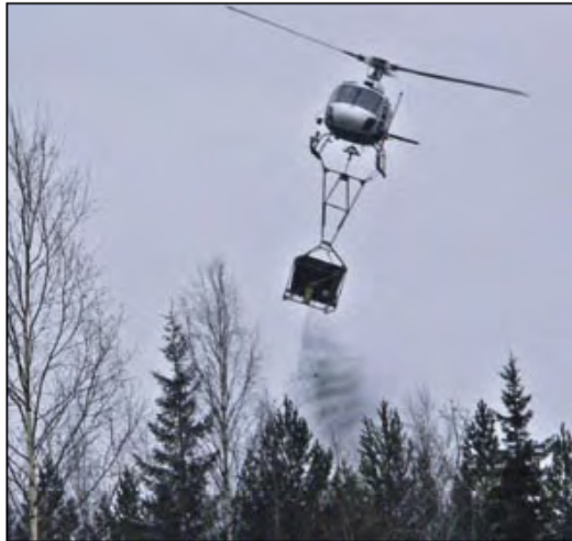
Figure 5: Ash spreading by helicopter [17]
