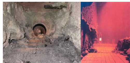
Figure 13: Examples for slag formation
