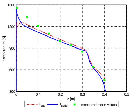
**Figure 3:** Axial profiles of solid and gas phase temperatures
