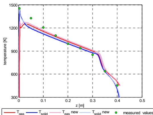
**Figure 7:** Axial profiles of solid and gas phase temperatures
