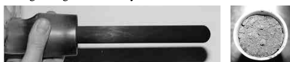
Figure 4: Cold finger with precipitate and ash sample after glowing condensation sludge in N 2
