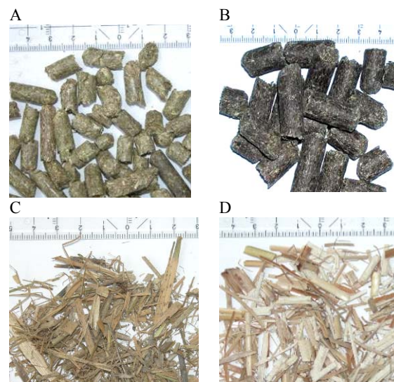
Figure 1: Fuels investigated: A) pelletised switchgrass (SG), B) pelletised cardoon (CA), C) chopped giant reed (GR), D) chopped miscanthus (MI)
