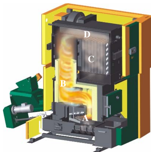
Figure 4: 150 kW th pilot-scale combustion plant used for the test runs Explanations: A...rotating grate, B...cyclone burner, C...boiler with automatic cleaning, D...location for deposit probe measurements
