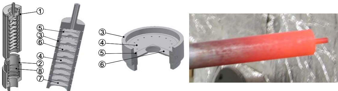
Figure 2: Scheme of the high-temperature impactor (HTI) (left) as well as HTI directly after a measurement (right)
