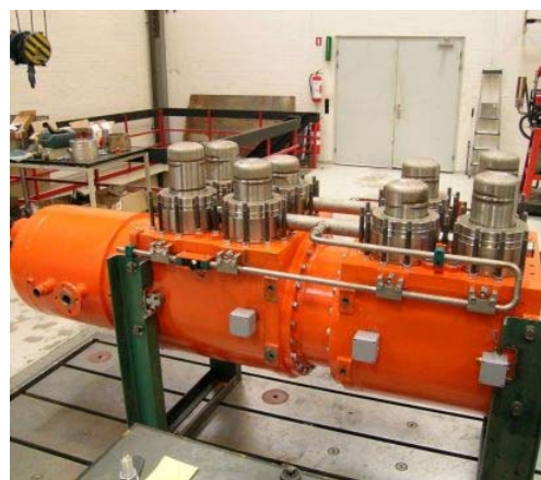
Figure 1: Picture of the 75 kW el Stirling engine (Stirling engine heater not mounted)
