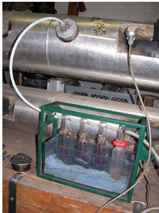
Flue gas sampling and gas scrubbing for the determination of SO x , HCl, NH 3 , Hg und gaseous heavy metals in the flue gas
