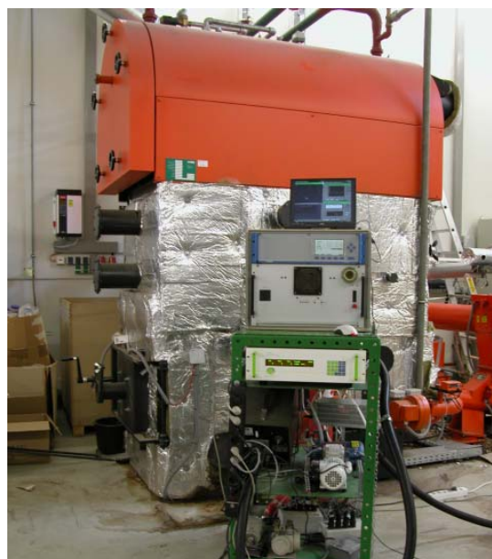
Flue gas analyses in operation at the pilot-scale combustion plant
