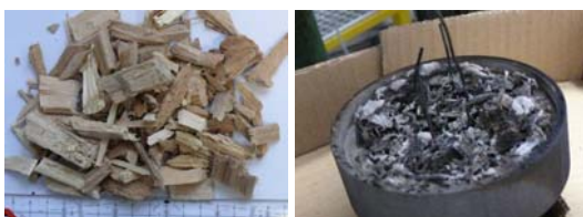
Fuel and residues (ashes) from a test run with beech wood chips
