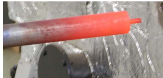
High temperature impactor immediately after sampling
