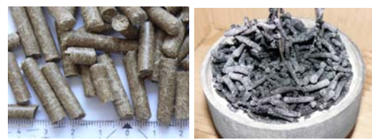
Fuel and residues (ashes) from a test run with straw pellets
