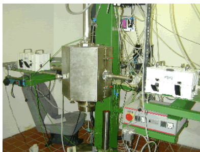
Reactor including process control and in-situ FT-IR spectrometer
