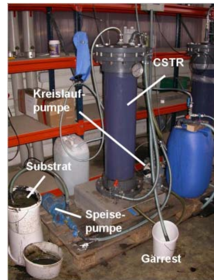
CSTR Pilotanlage (CSTR: continuously stirred tank reactor)
