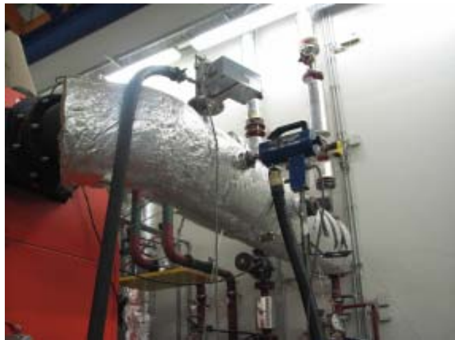
Gas sampling during a test runs at a biomass pilot-scale combustion plant
